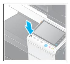
When the **Power** key is pressed, the status of this machine changes as shown below. The way status changes varies depending on how the **Power** key is pressed.
